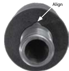
Figure 29b - Reinstalling Nozzle Protector
