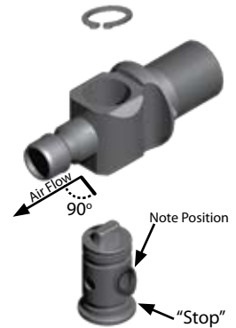
Figure 29a - Reinstalling Nozzle Valve Plug
