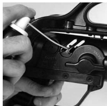
Figure 27b - Lubrication of Mechanism with Corrosion Block
