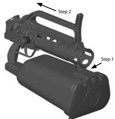
Figure 10b - Disconnecting Launcher from Line Container
