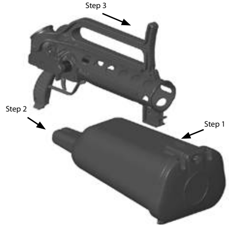
Figure 10a - Connecting Launcher to Line Container
