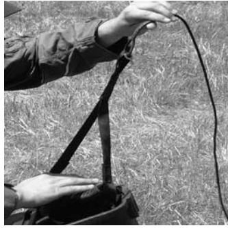
Figure 22b - Leave the Tether out of the Line Container
