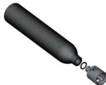
Figure 27a - Cylinder and Nozzle Assembly
